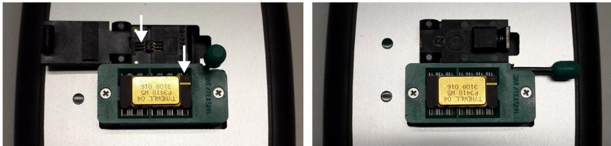
**Figure 4:** Device positioning – sockets open (left), sockets closed (right). Arrows indicate Pin 1.
