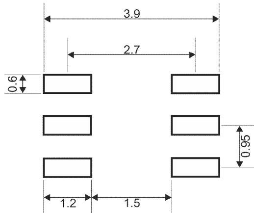
**Figure 6:** Recommended solder pad layout. All dimensions are in millimeters. Note the drawing is not to scale. Dimensions are inclusive of plating.
