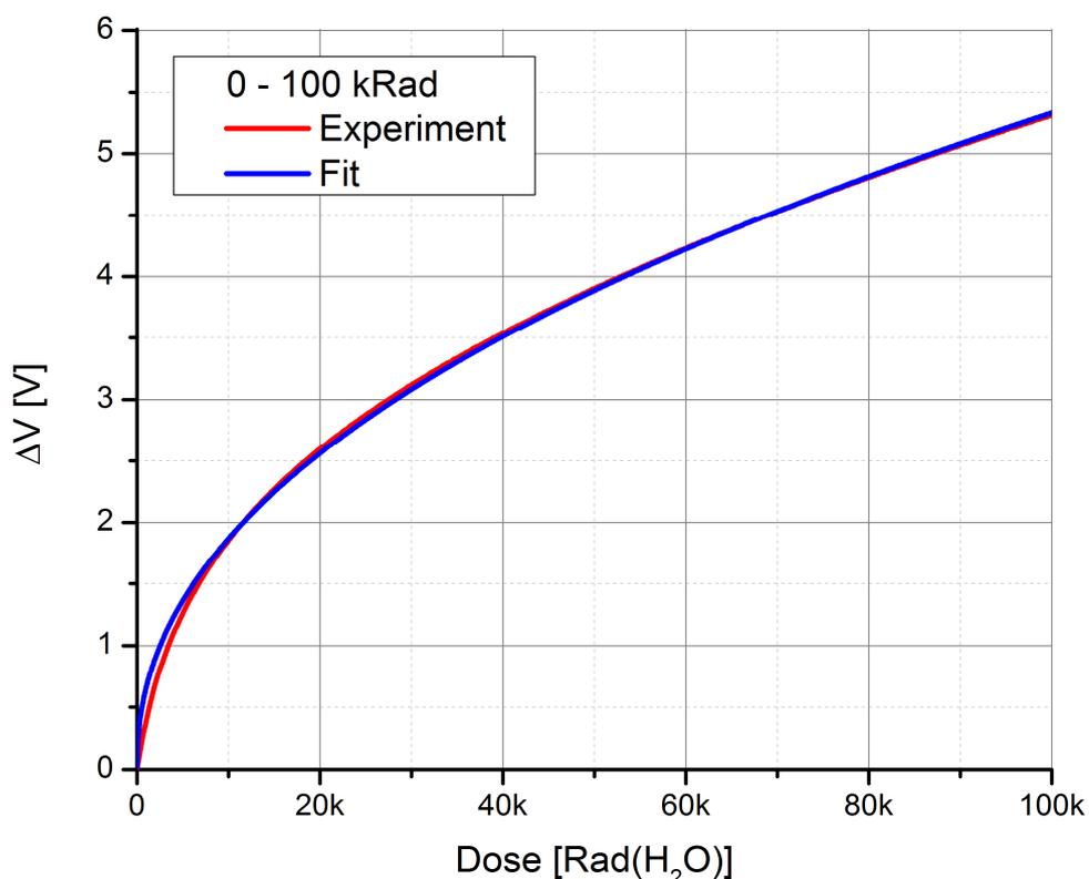
**Figure 4:** Typical calibration curve indicating change in RC\_V during irradiation. Irradiation at room temperature with Co-60 gamma source, dose rate ~50 Gy/h (5 krad/h).. Voltage measurements performed at room temperature using 0.2% duty cycle with all terminals grounded between measurements
