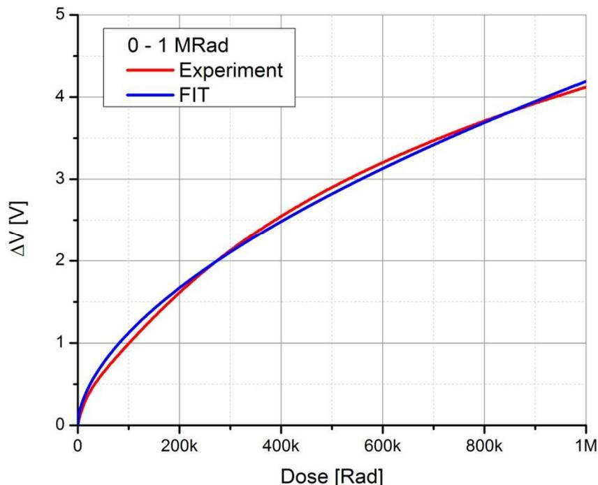
**Figure 4:** Calibration curve indicating change in RC\_V during irradiatio. Irradiation at room temperature with photon source, dose rate ~500 Gy/h (50 krad/h). Voltage measurements performed at room temperature using 0.2% duty cycle with all terminals grounded between measurements
