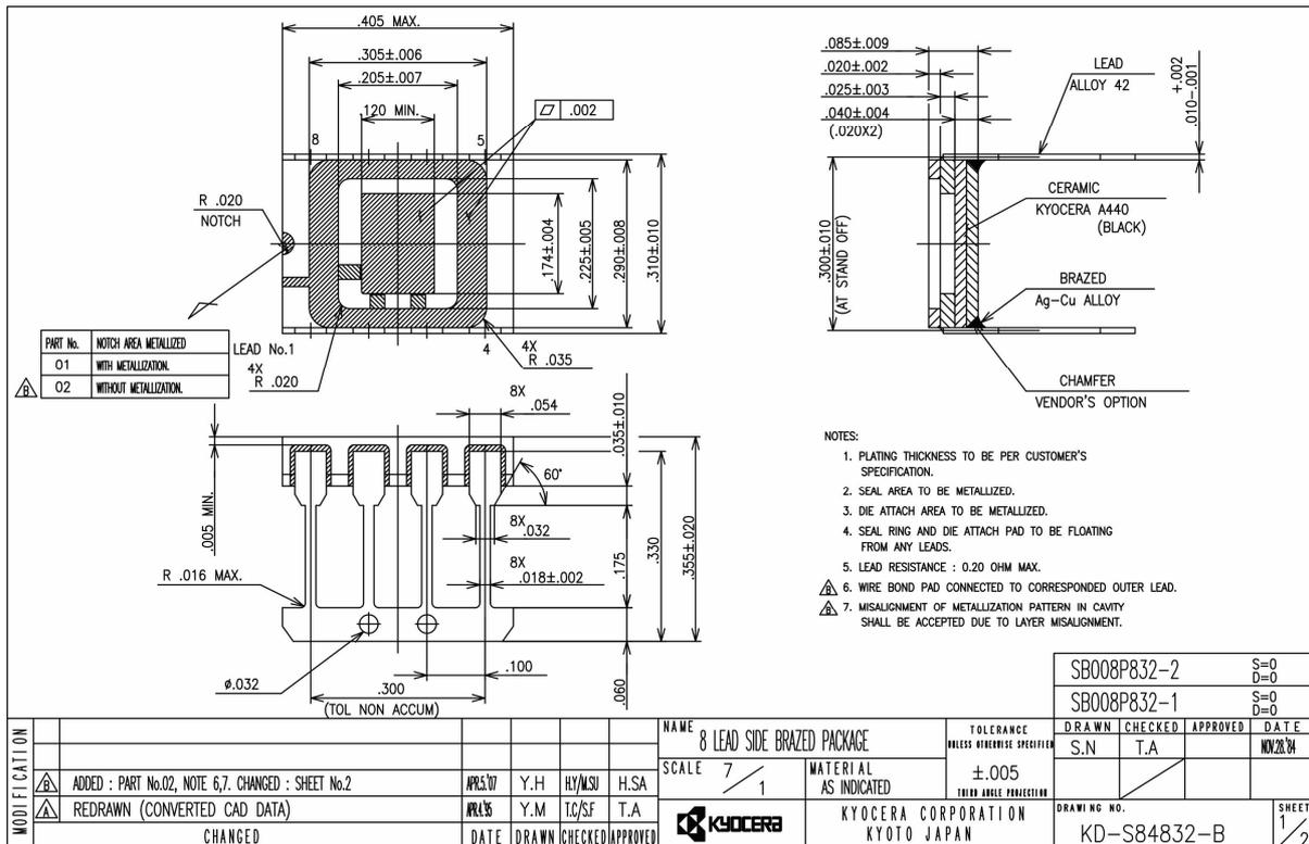
**Figure 5:** VT06 package diagram.
