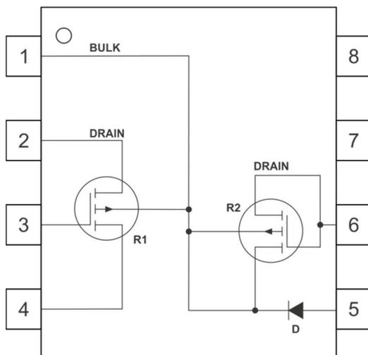
**Figure 1:** VT06 pin-out drawing.
