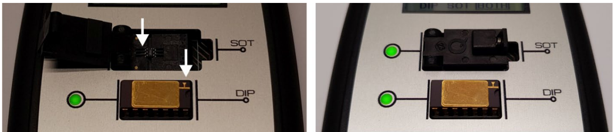
Figure 4: Device positioning – sockets open (left), sockets closed (right). Arrows indicate Pin 1.
