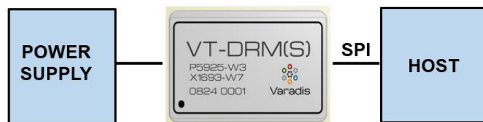
Figure 18: SPI connection with HOST.
