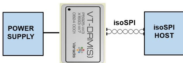
Figure 19: isoSPI connection with HOST.
